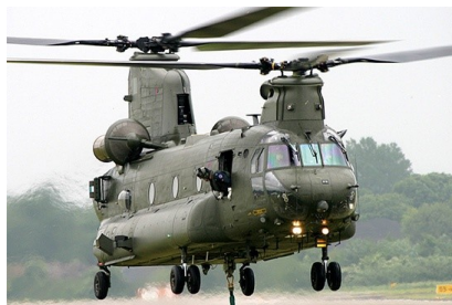
No Tail ( Double Main Rotor )
