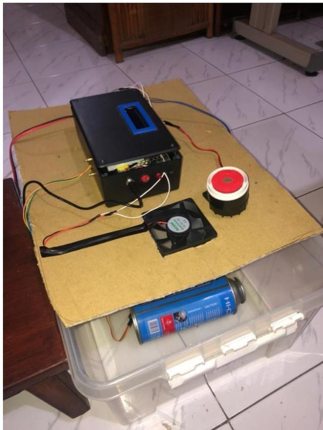
Gambar 5. 4 Prototype Monitoring Gas
