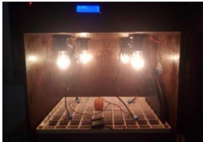
Gambar 2. 3 Inkubator Telur Ayam (Sumber: Noor et al., 2019)
