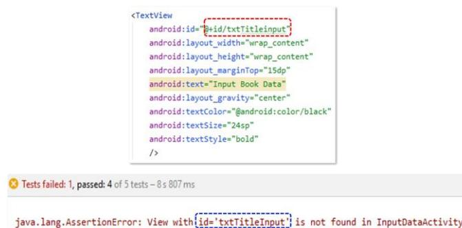
Gambar 4. 8 Failed Test
