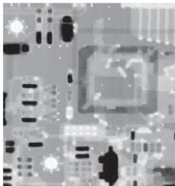
Gambar 2.8 *Grayscale Image* Setelah Proses *Closing*
