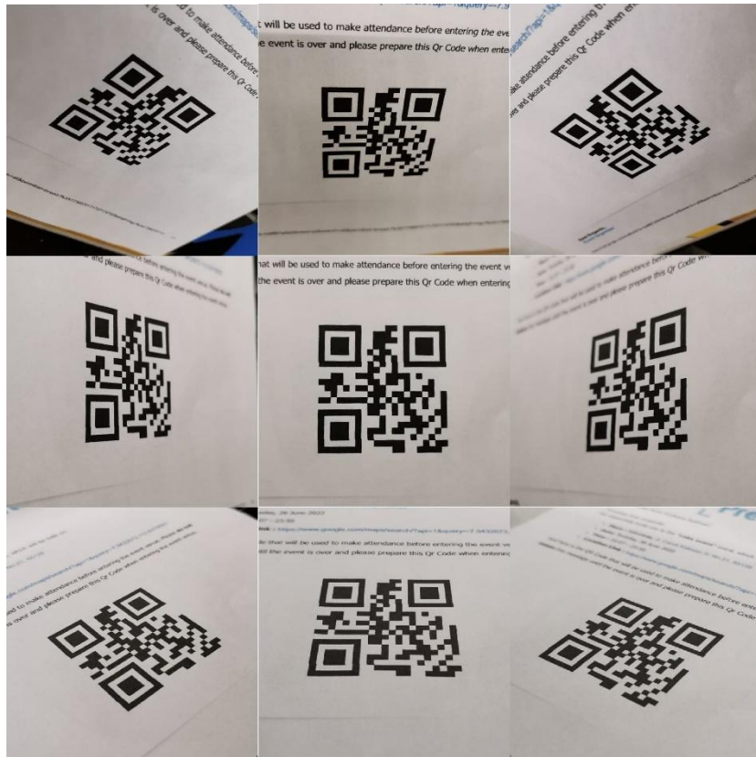
Figure 5.45 Different Angles of Scanning the Printed QR Code with Warm Ambient Light Turned to 50%
