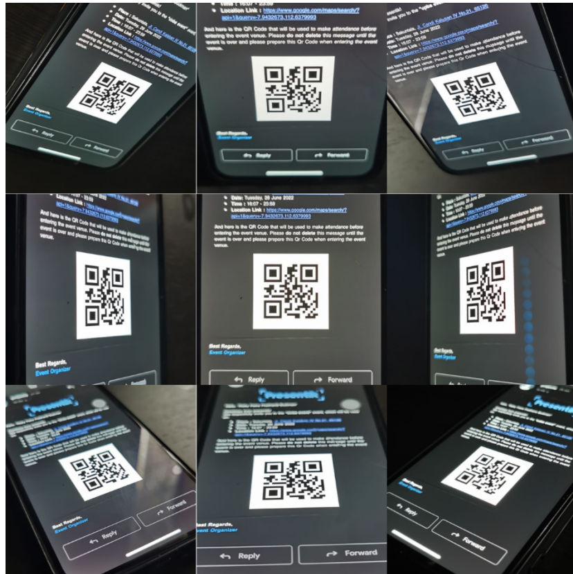
Figure 5.43 Different Angles of Scanning the QR Code with Phone Brightness Turned to 100%
