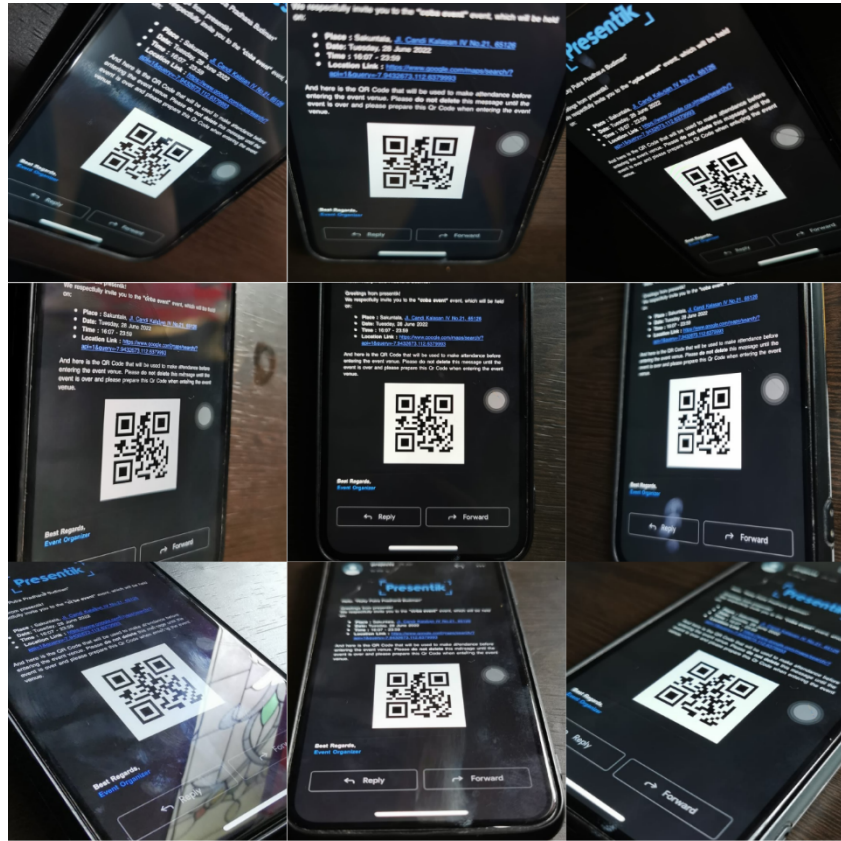
Figure 5.40 Different Angles of Scanning the QR Code with Phone Brightness Turned to 25%
